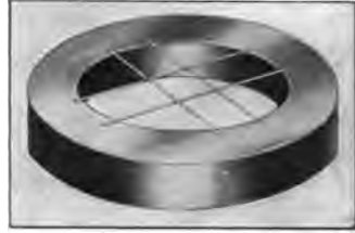
Fig. 90.—Diaphragm of eye-piece showing hairs in position (Miller).
